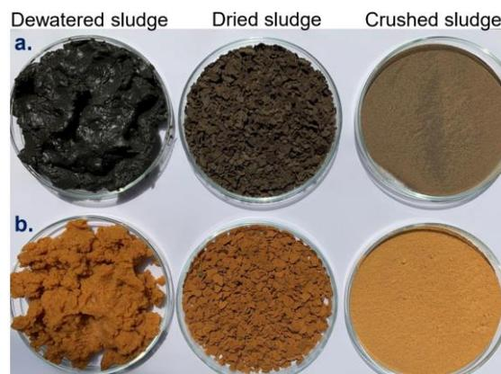
Fig. 1: a. Bio-sludge and b. Che-sludge pre-treatment
