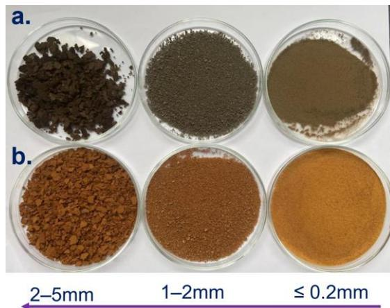
Fig. 2: a. Dried bio-sludge and b. dried che-sludge: different particle size
