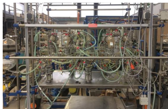
Fig. 2: Five-stage mixer-settler battery available in the laboratory
