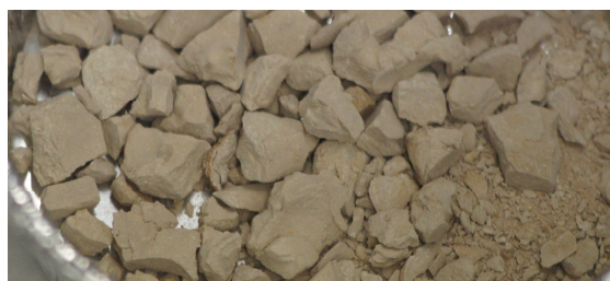
Fig. 4: precipitate obtained by PULSE process containing CaP salts
